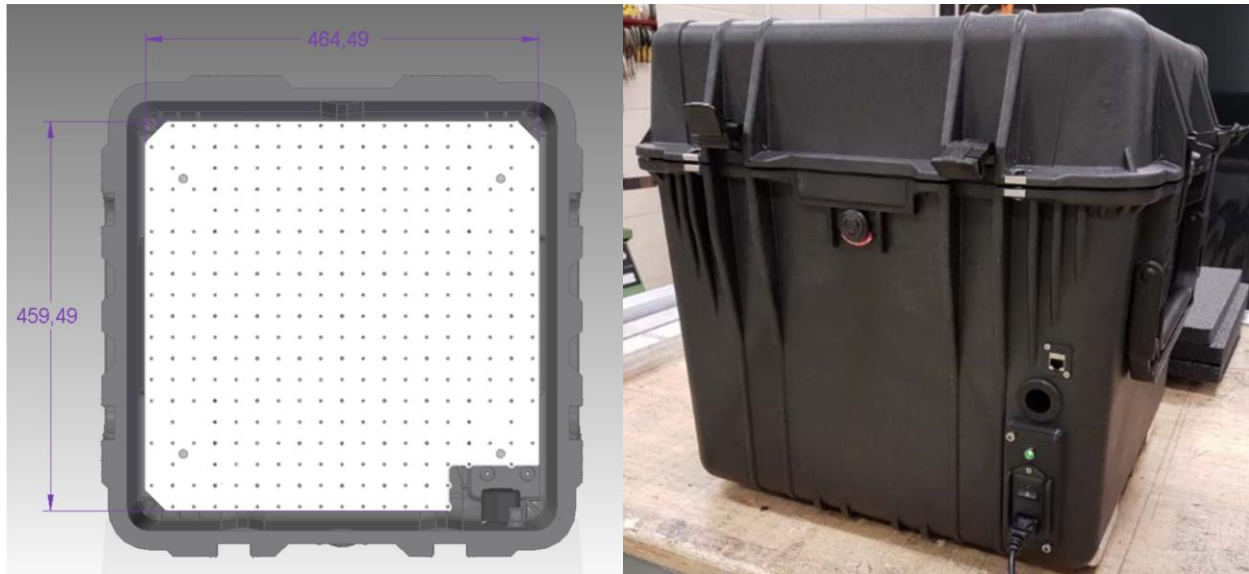
Figure 1: (a) Pelican case interior mounting plate with dimensions 459.49 x 464.49 mm. (b) Pelican case exterior with modifications (bottom-right corner)
